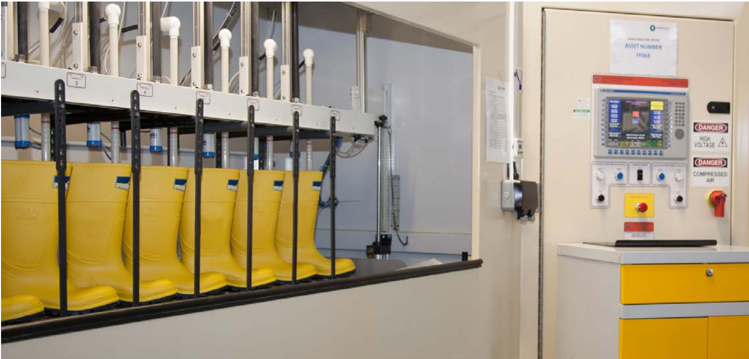
Dielectric boots under test at the Workmaster™ boot factory
